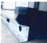
The Unit base is manufactured using 3mm folded galvanised sheet metal. The base heights can be customised from the standard 100mm to 400mm which can include a U Trap or plinth removal
